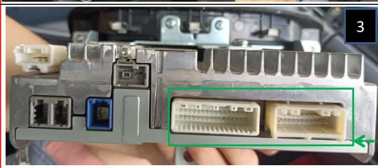
The Android cable is cross-connected with the car's original cable
