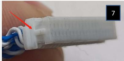
When installing, please pay attention to the correct connection of this interface, do not plug the reverse interface, and do not damage the contact pins of the interface
