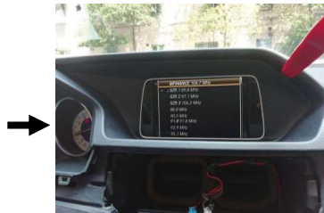
6. Pry out the decorative frame from the original monitor.
