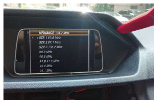
2.Pry out the frame of original monitor and remove the fixing screws
