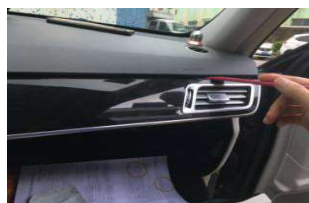
6.Pry the top buckles from the air conditioning vent.(Note:Fixed well the vent when prying the buckles)
