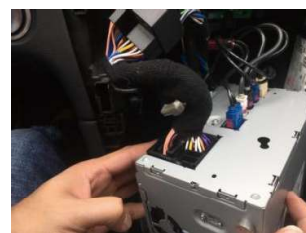
8.Remove the power harness from original host, and connect it to android harness.
