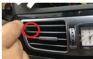
3.Pry the buckles on the left side of the air conditioning vent
