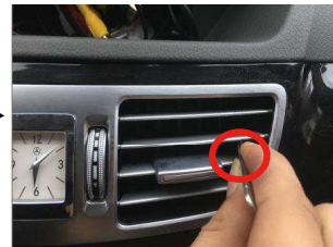
3. Pry the buckles on the right side of the air conditioning vent
