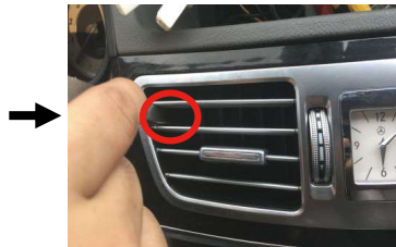
2. Pry the buckles on the left side of the air conditioning vent
