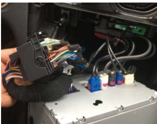
9. Remove the power harness from original host, and connect it to Android harness.
