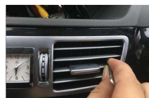
4.Pry the buckles on the right side of the air conditioning vent
