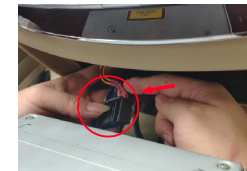
14. Connect the fiber optic cable you took out to the main cable of CarPlay
