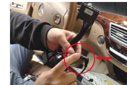
11. Take out the main cable of CarPlay, be careful not to unplug the docking plug on the main cable (the NTG4.5 host needs to be unplugged)
