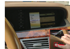
20. Enter the audio interface - choose AUX, Long press phone-ending button to switch to carplay interface. (If the original car does not have AUX, you need to activate the AUX of the original car first)
