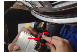
16. It is recommended to connect the main cable of CarPlay to the host in the last step
