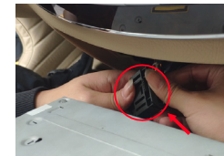
13. Connect the main line of CarPlay with the main line of the original car
