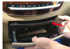
4. Remove the center console
