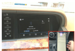
21. Turn on WiFi on the phone, keep it on, then turn on Bluetooth, search for and connect CarPlay Bluetooth (You can enter the Bluetooth interface in the CarPlay system to view information such as the name of the CarPlay Bluetooth)
