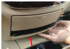
1. Remove the trim panel under the center console
