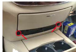
2. Unscrew the screws on the bezel console
