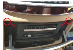
3. Open the center console, then open the small shutter of the screw; unscrew the screws
